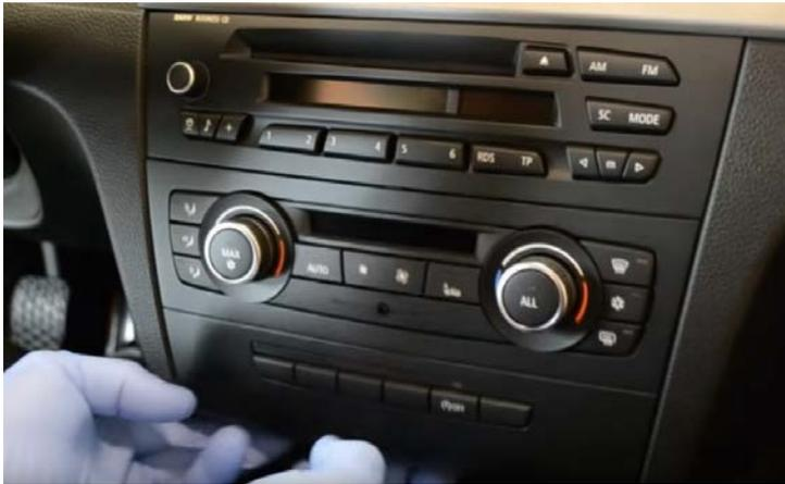
1. Pull the cover of the air conditioning control unit on the lower side slightly forward to release it from the multimedia control unit.
