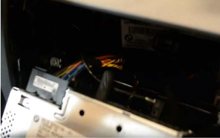
4. To be able to completely remove the device from the device slot, you have to disconnect first all plug connections (e.g. main connection cable, antenna cable, etc.) on the back of the device.
