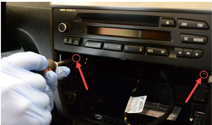
3. Use a screwdriver to loosen the two fastening screws on the side of the original radio.
