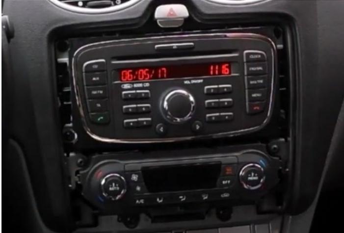
2. Using a Phillips screwdriver, loosen the four mounting screws of the original radio.
