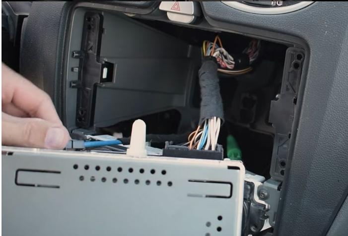
3. In order to be able to completely remove the device from the device slot, you must first disconnect all plug-in connections (eg main connection cable, antenna cable, etc.) on the back of the device.
