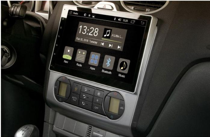
5. Neatly arrange the wires to the side, making room for the Radical device. Carefully slide it into the radio slot. Push back the R-C10FD2 until you hear the clicking sound of the latching mechanism.
