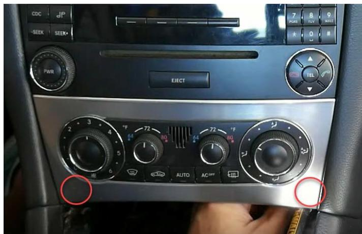
3. Now you have to loosen the brackets for the cover in the center console. For this you need a thin, long slotted screwdriver. After you have loosened the clips, you can pull all the plugs off the controls.
