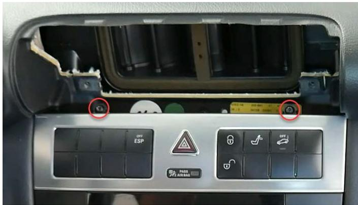
5. Now loosen the two screws of the climate control with a Torx screwdriver.
