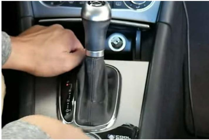
1. First you have to carefully pull out the cover in the center console. This is only attached and not screwed. It is best to start in the area of the ashtray and then carefully pull the part out at the top. The sleeve of the gear knob can be easily pulled out upwards.
