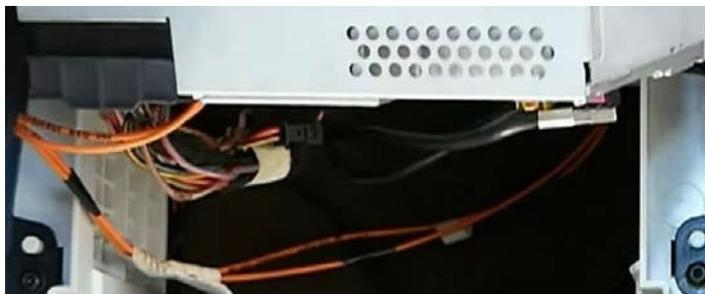
7. Carefully pull the original radio out of the shaft at the necessary speed. Make sure that you do not damage the cables. Remove the cables one at a time and carefully, make sure that the cables do not fall back into the slot.
