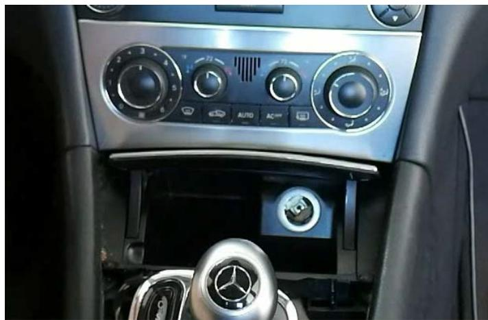
2. You can now easily remove the ashtray by pushing the two rakes away from the ashtray, as can be seen in the picture.
