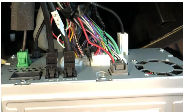
5 Disconnect individually all cable connections shown here to the original radio.
