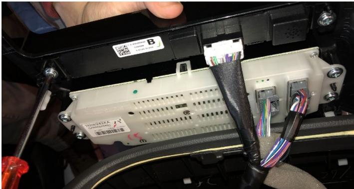
2 Disconnect the cables and remove the top two screws from the climate control unit to disconnect the radio and the clutch
