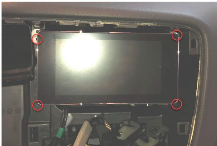
4 Loosen the four screws on the radio. You release the radio from the frame anchorage and can then pull it out of the shaft
