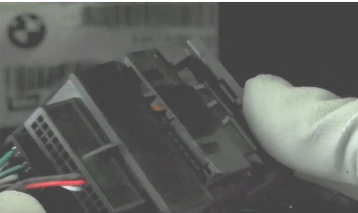
3. Connect the respective main connection cable (# 11) of the Radical device (# 1) to the plug of the vehicle and close the locking mechanism of the connector. Then connect the CAN-BUS interface (No. 12) to the main connection cable. Connect all cables previously routed in the radio slot and the original antenna cables to the Radical unit (# 1).
