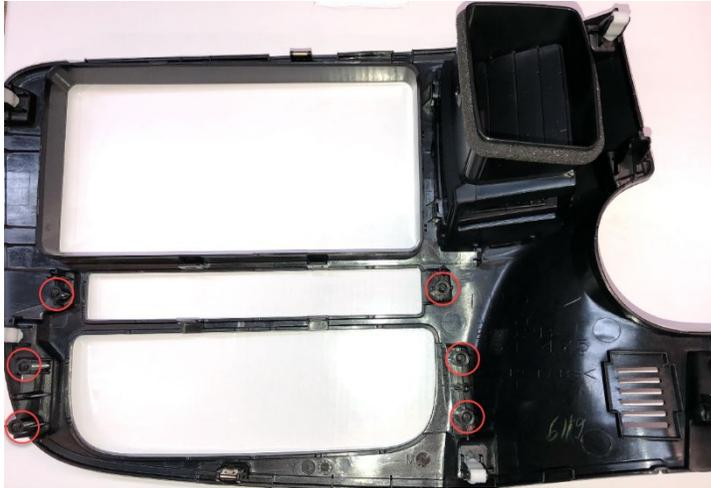
3 Now remove the red marked screws from the plastic frame so that you can remove the climate control and the ECO indicator from the frame.
