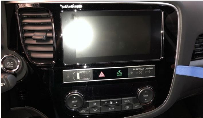
1 From the right side, carefully pry the plastic frame surrounding the original device out of its moored anchorage. Use the supplied plastic unlocking tool for this step. Run the unlocking tool once counterclockwise around the plastic frame. The plastic frame should now be completely detached. Loosen and remove the four Torx screws (T25) from the original device.
