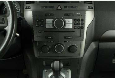
2. It should be possible to pull out the radio without applying brute force.
