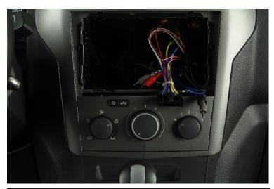
6. Connect the main harness (No. 11) of the Radical device (No. 1) to the Fakra connector of the car and close its locking mechanism. Connect the CAN bus interface (No. 12) to the main harness. Connect all the cables to the Radical device (No. 1), and the original antenna cables.
