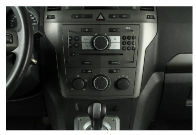
Unlock the OE radio with the unlock tool (No. 14) contained in the set. You need to insert two keys.
