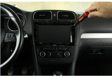
Neatly arrange the wires to the side, making room for the ZENEC system. Carefully slide it into the radio slot and fix it in place, using the four original Torx screws.
