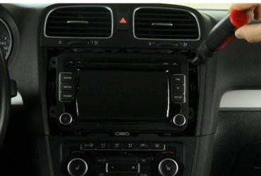
2. Set the prying tool anticlockwise around the trim frame, to release it from the console. The trim frame should come off of the console completely. Unscrew and remove the four Torx screws (T25) of the original device.
