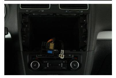
3. Remove the original device by pulling it out of the radio slot. Disconnect all the cables from its backside.
