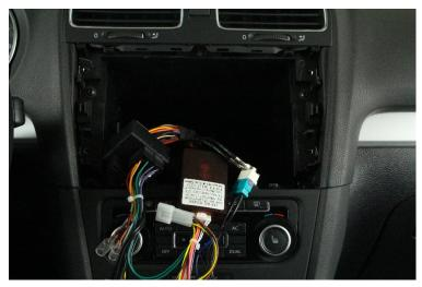
6. Connect one of the main connection cables (No. 11) of the Radical device (No. 1) to the Plug connector of the car and close its locking mechanism. Following this, connect the CAN bus interface (No. 12) to the main connection cable. Connect all the cables to the Radical device (No. 1) those previously run in the radio bay and the original antenna cables.
