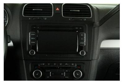
Gently lift the trim frame starting on the right side of OE device. Use the supplied plastic removal tool for this step.
