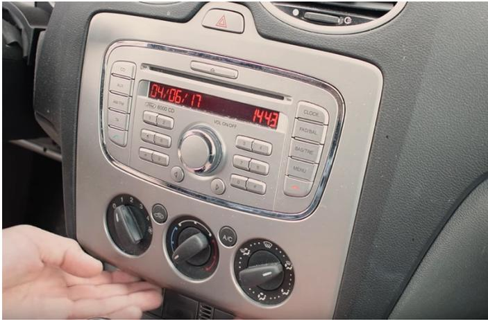
1. Pull the plastic frame slightly forward on the bottom side to release it from the multimedia control unit.
