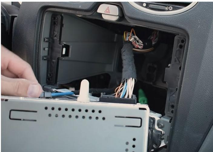
3. In order to be able to completely remove the device from the device slot, you must first disconnect all plug-in connections (eg main connection cable, antenna cable, etc.) on the back of the device.
