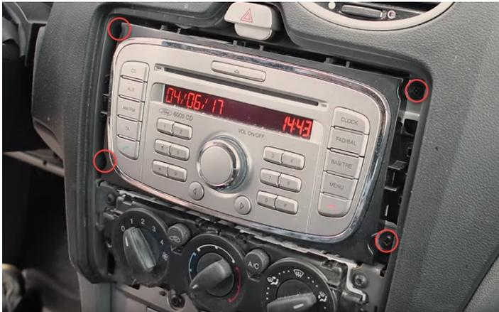
2. Using a Phillips screwdriver, loosen the four mounting screws of the original radio.
