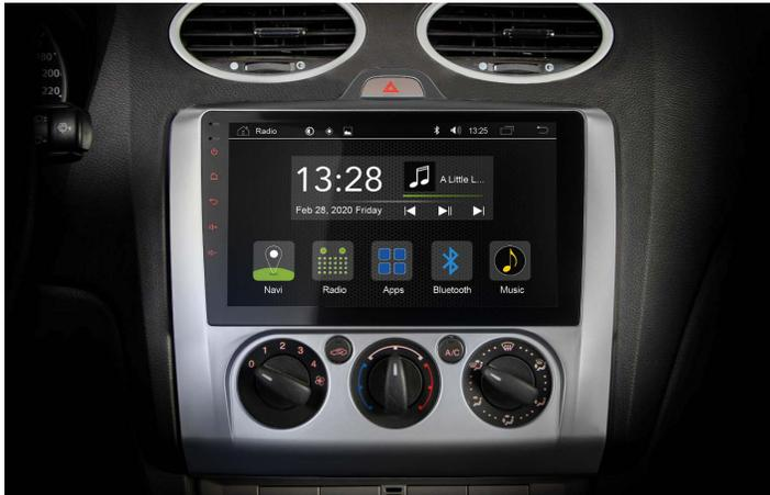
7. Neatly arrange the wires to the side, making room for the Radical device. Carefully slide it into the radio slot. Push back the R-C10FD1 until you hear the clicking sound of the latching mechanism.
