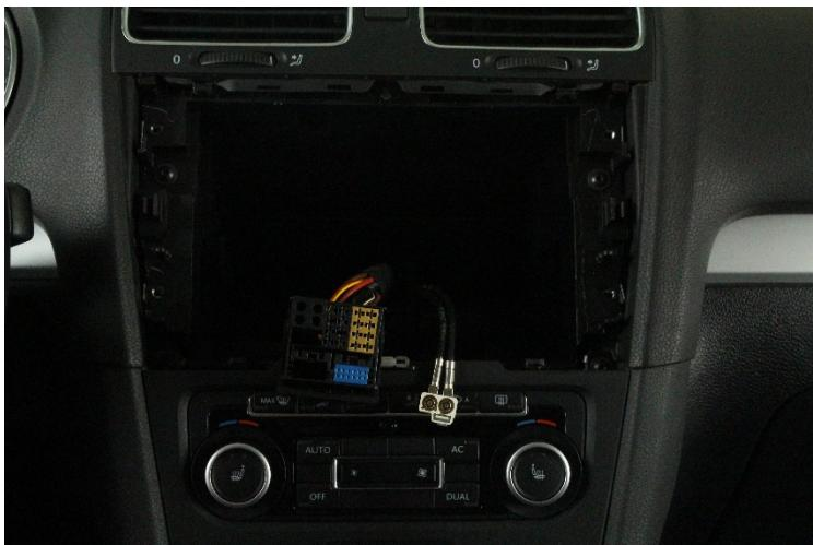
1. Gently lift the trim frame starting on the right side of OE device. Use the supplied plastic removal tool for this step.
