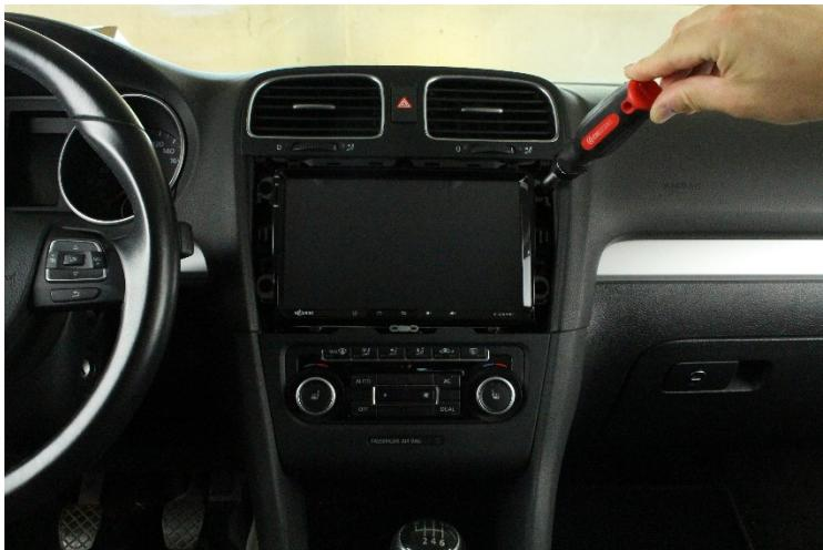
7. Neatly arrange the wires to the side, making room for the ZENEC system. Carefully slide it into the radio slot and fix it in place, using the four original Torx screws.
