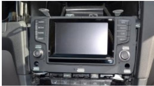
6. Use the removal tools included in the package (No.15), to remove the EO head unit. Once done, unlock all connectors on the backside and remove the OE radio completely.
