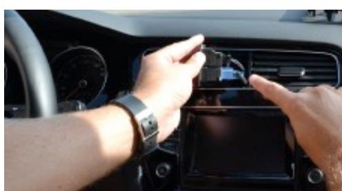
4. Take out the switch panel to remove the radio front panel.
