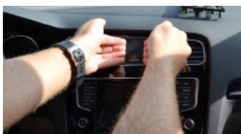
3. Next, pull out the switch panel with the button for the hazard flasher to unlock the connecting plug.
